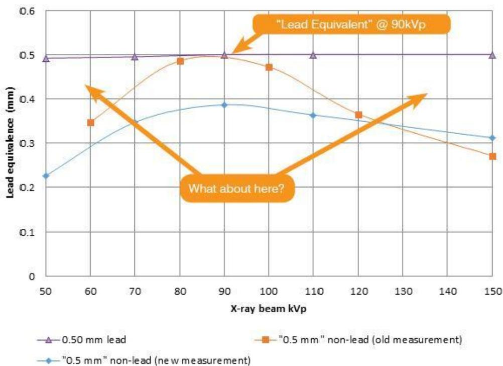
This graph perfectly illustrates the missing picture. It is made from a set of real data of a non-lead material's lead equivalence plotted against the x-ray beam kVp and compared against a lead-based material. The key thing to note here is that **while the non-lead material is equivalent to lead at the 90 kVp mark, it drops off at lower and higher energies.** Manufacturers can get away with claiming a 0.5mm lead equivalence but this shows what is really happening.
