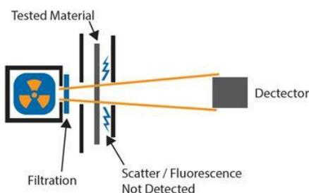
**Shows how secondary scatter is missed and not shown in test results.**
